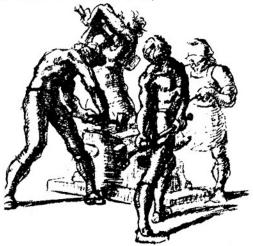
The rough thinned plate was cut into pieces, heated again and hammered then into shape on small anvils, called stakes. There were different shaped stakes for the shaping of various parts of the armon.
